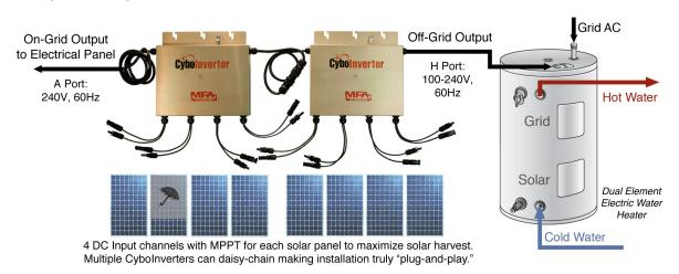
The following graphic shows a 4-channel 1.2KW On/Off-Grid CyboInverter that has an ongrid AC output port and an off-grid AC output port. Each inverter has four input channels that can connect to four 300W DC sources including solar panels, wind generators, or batteries and produce 1150W AC peak power. Each input channel has its own control and MPPT to eliminate solar partial shading problems and maximize power production. The product is patented, UL1741 certified,
